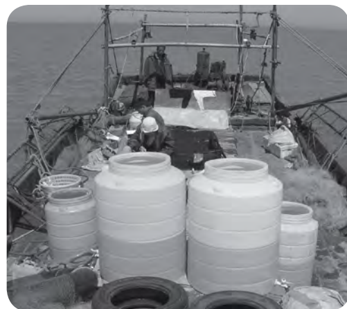
Collecting water from the Yellow River estuary for analysis of radium isotopes. Over 100 liters of muddy water must be processed for each analysis. Radium isotopes can be used to determine exchange rates of estuarine waters with ocean waters.
